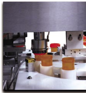
Close-up of capping area
